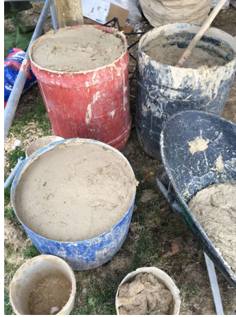
Clay mixed with some sand and small pieces of chopped straw
