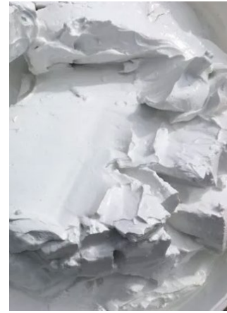
Lime putty ready to apply to walls
